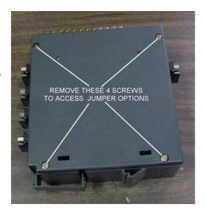
Separate the case to access the jumper options. The silkscreen on the printed circuit board summarizes the jumper options as detailed in the following paragraphs.
