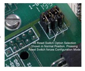
affect. If J8 is in the 2-3 position, then pressing the Reset Switch will cause the Omnii-Comm™ to perform the same actions that it would on a power up cycle. This usually is a cold start. All RAM memory will be cleared, Power On Self Tests will be run, the Log-on messages will be sent out and polling will be started. The Configuration mode will NOT BE ENTERED.
