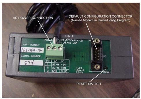
handshake lines RTS and CTS. The photograph at right shows an AC power connection option (-1YZ).
