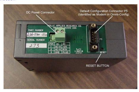
to its "Configuration Mode". All normal operation will be suspended and the Default Configuration Connector, in this case the P5 connector, will be reconfigured from whatever it was doing previously to a "Configuration" connector at 9600, 8, N, 1 in preparation for talking with the Omnii-Config™ program.
