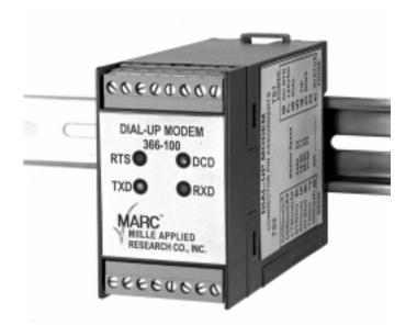
The MARC™ Model 366-100 is a full-function dialup modem that mounts on a standard DIN-rail and provides data communications with other Bell and CCITT compatible modems at speeds up to 33.6K baud.
